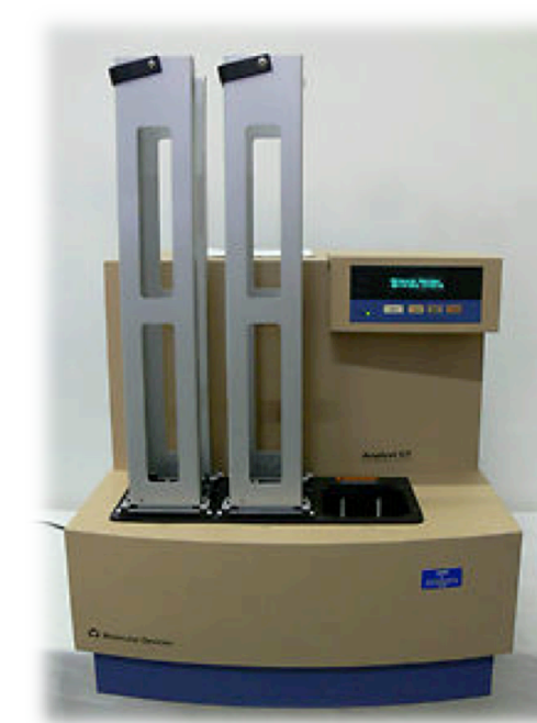
Figure 2. Process Growth Curves. 96 well plates are run on instrument (right) for 32hrs. OD600 nm is recorded every 30mins to produce growth curve (above). Parameters are captured to fit to a logistic model, which is then used to determine growth level.
